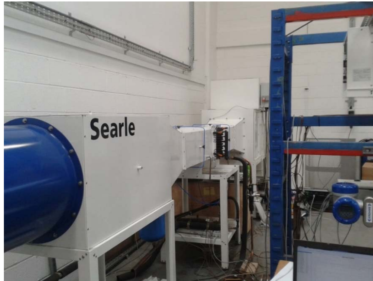
Figure 2 - Condenser Coil in External Heat Transfer Rig
